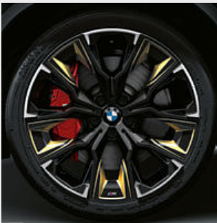
□ 20" M aerodynamic wheels 920 M Multicolour with Gold accent and run-flat tyres, gloss-lathed, wheel size 8J x 20 with 225/40 R20 tyres. 4,6,*
