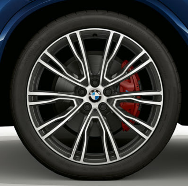
□ 21" BMW Individual light alloy wheels V-spoke style 726 I Bicolour, Orbit Grey with mixed tyres and run-flat tyres, gloss-lathed, wheel size front 8.5J x 21 with 245/40 R21 tyres, wheel size rear 9.5J x 21 with 275/35 R21 tyres.
