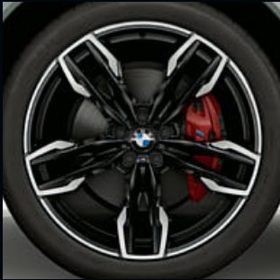
□ 21" M light alloy wheels Double-spoke style 718 M Bicolour Jet Black with mixed tyres and run-flat tyres, gloss-lathed, wheel size front 8.5J x 21 with 245/40 R21 tyres, wheel size rear 9.5J x 21 with 275/35 R21 tyres.
