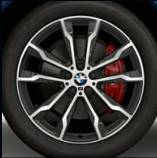
■ 20" M light alloy wheels Double-spoke style 699 M Bicolour Orbit Grey with mixed tyres and run-flat tyres, gloss-lathed, wheel size front 8J x 20 with 245/45 R20 tyres, wheel size rear 9.5J x 20 with 275/40 R20 tyres.
