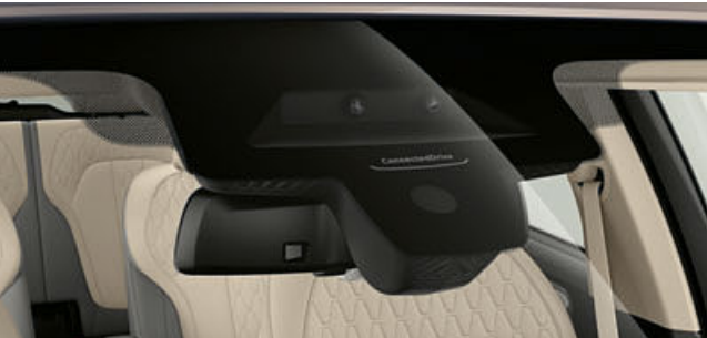
The standard High-beam Assistant supports driving in the dark by automatically adjusting the headlights in response to oncoming traffic or vehicles up ahead. Where there is sufficient ambient light, for example in built-up areas, it reacts by automatically switching off the high-beam.
