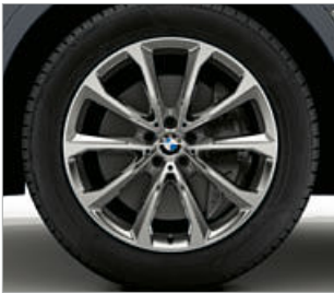
20" light alloy wheels V-spoke style 750 Reflex Silver with run-flat tyres, wheel size 8.5J x 20 with 275/50 R20 tyres.
