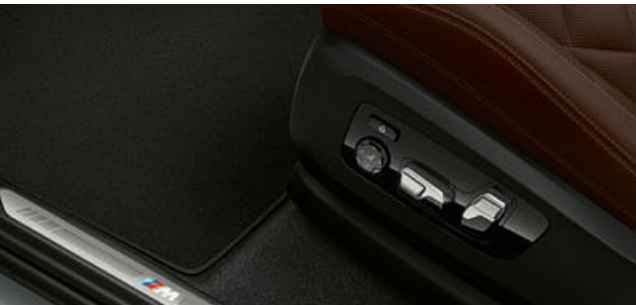
The standard electric seat adjustment with memory function allows the desired settings for seat, exterior mirror and steering wheel to be stored.
