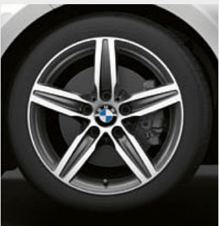
□ 17" light alloy wheels Star-spoke style 379, Orbit Grey, gloss-lathed, 7.5J x 17 with 225/45 R17 tyres.
