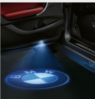
○ When the doors are opened, one of a choice of four graphics is projected on the ground adjacent to the vehicle, for perfect illumination of the entry area.
